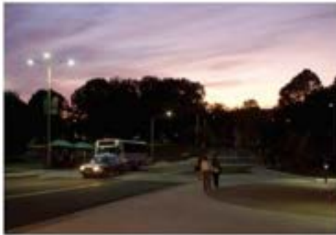
Figure 4-5. A street located in an LZ-2 area: fully shielded lighting, uniform distribution. (Image courtesy of Bob Parks)
